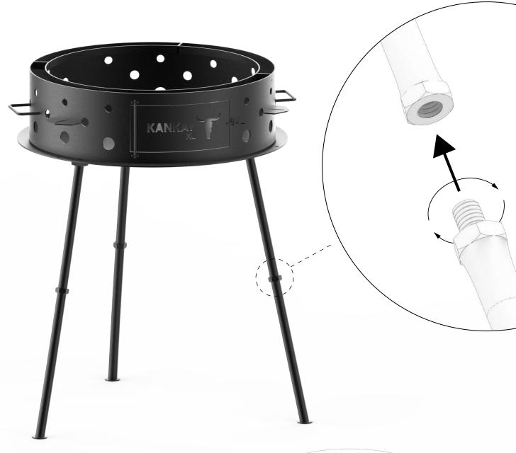
Each leg is divided in two sections. Screw them together, then screw the whole leg to the bottom of the disc plow.
