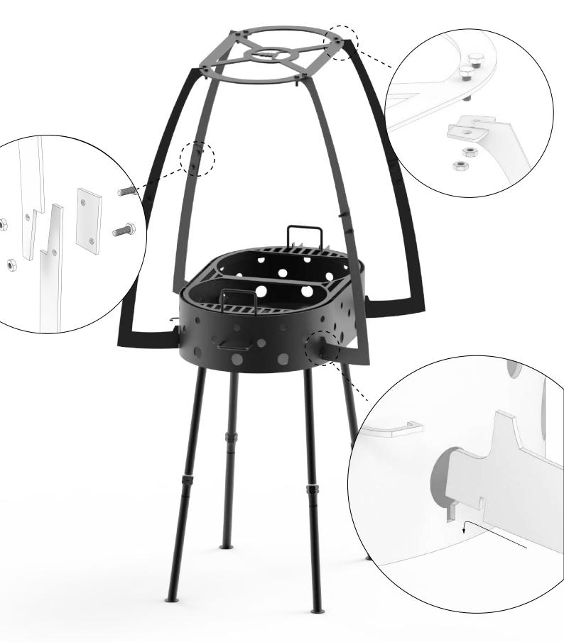
Mounting the cage is all about locking in the components
